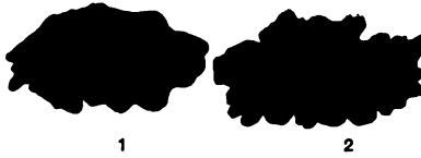
CONTACTS OF 48 \frac{1}{2} -IN. STEEL-TIRED TRAILER TRUCK WHEEL, ATLANTIC LOCOMOTIVE. WEIGHT ON WHEEL, 19,210 LBS.
